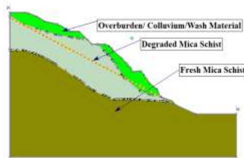
Fig. 13 Initial profile before excavation with colluvium up to certain depth
