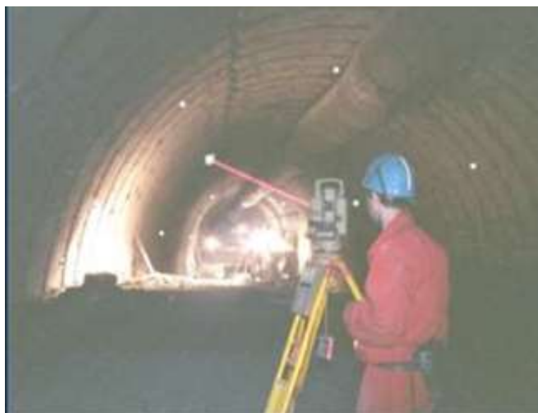
Fig. 11 : Measurement of radial tunnel deformation
