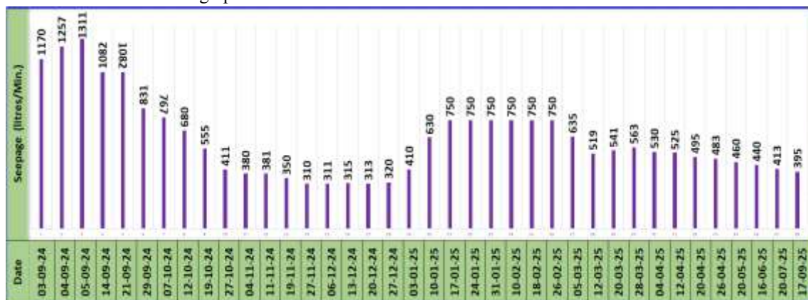
Graph A- Seepage Trend in Machine Hall during and after remedial measures
