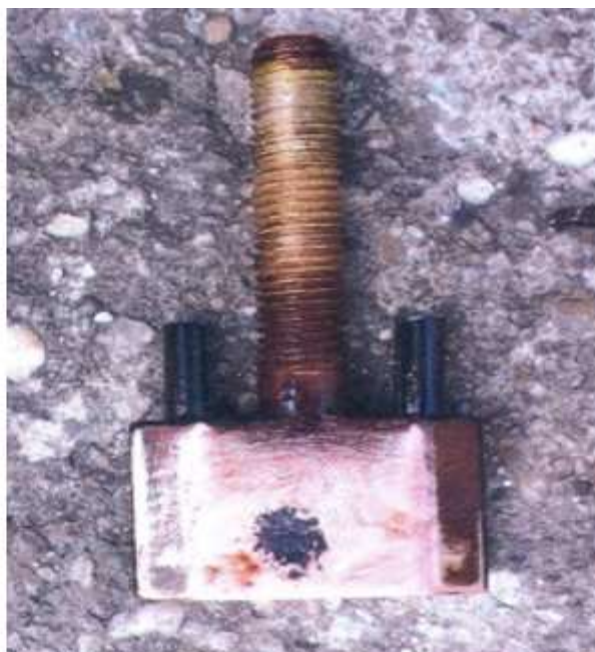
Fig. 4 : Pitted Male Tap Changer Contact (Tap No. 3 - 1W Phase)
